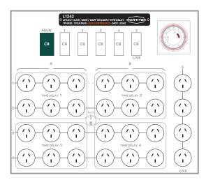
LMU with 32 timed + 4 live sockets. 16ON/16OFF operation with Time Delay to stagger ignition of lamp sockets when turning on.
