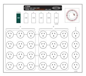
LMU with 24 timed + 4 live sockets. 12ON/12OFF operation with Time Delay to stagger ignition of lamp sockets when turning on.
