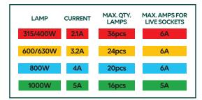
• If using 600/630W lamps, the maximum number of lamps allowed to this LMU's timed sockets are 24pcs and 6A maximum for the live sockets.
