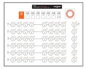
LMU with 48 timed + 6 live sockets. 24ON/24OFF operation with Time Delay to stagger ignition of lamp sockets when turning on.
