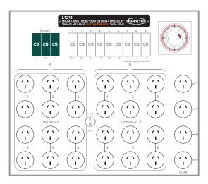
LMU with 24 timed + 4 live sockets. Selectable 12ON/12OFF or 24ON operation with Time Delay to stagger ignition of lamp sockets when turning on.
